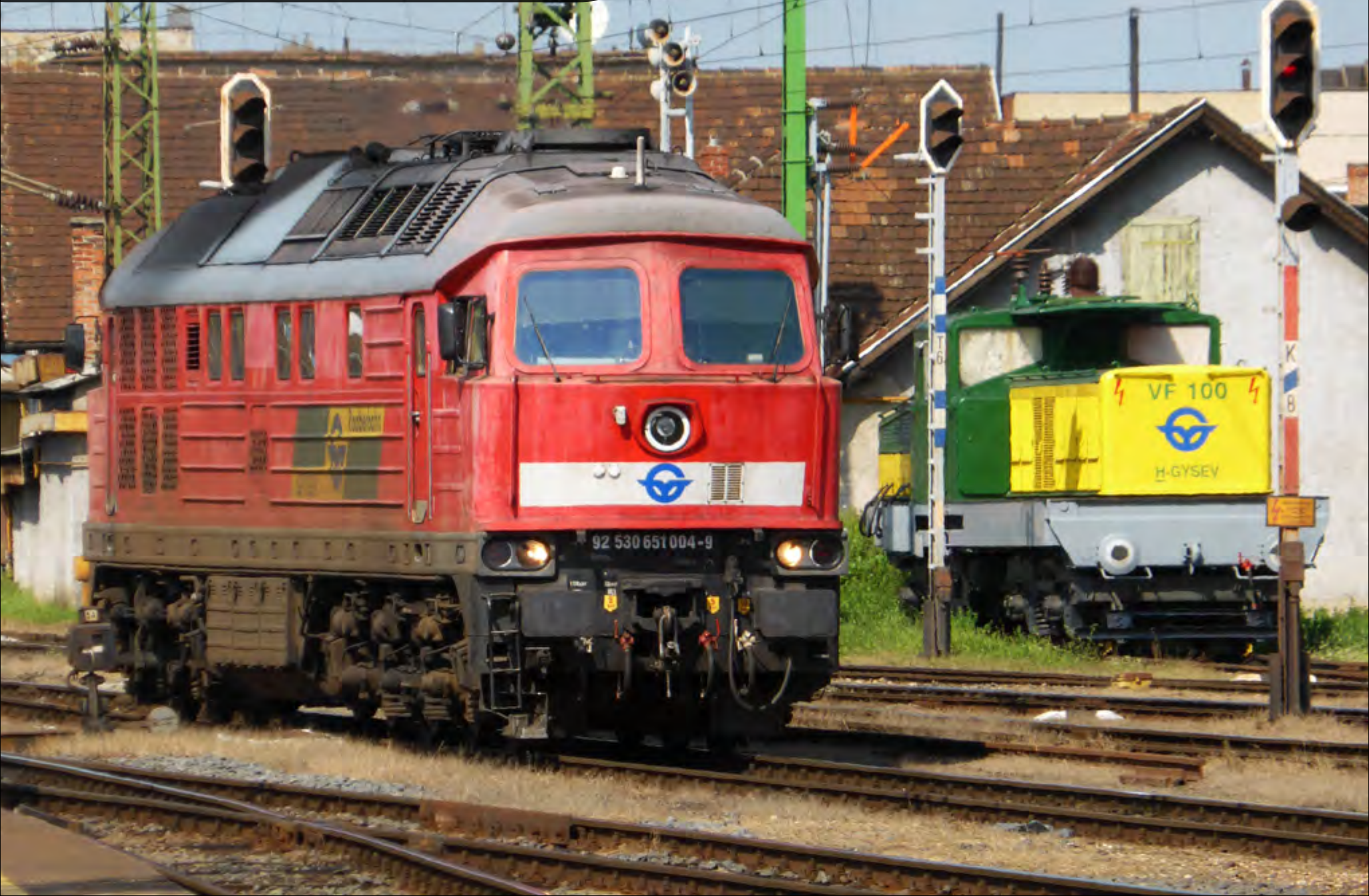
GYSEV's Class 651.004 is seen at Szombathely passing Sopron transformer unit VF100 which was originally V42.529 until withdrawal in August 1987. The Sopron transforms current from the 25kV overhead which is used to pre-heat coaching stock as well as other electrical requirements . Steamsounds
